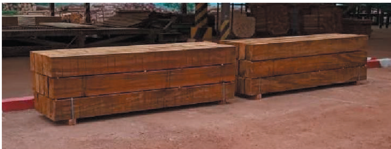
Sleepers made of Okan (photo: Frédéric Viroux, Pallisco, Cameroon)
