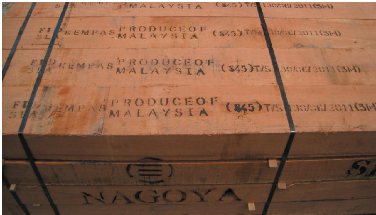
Sleepers made of Kempas (photo: Benoit Gomet, France Timber, Nagoya, Japan)
