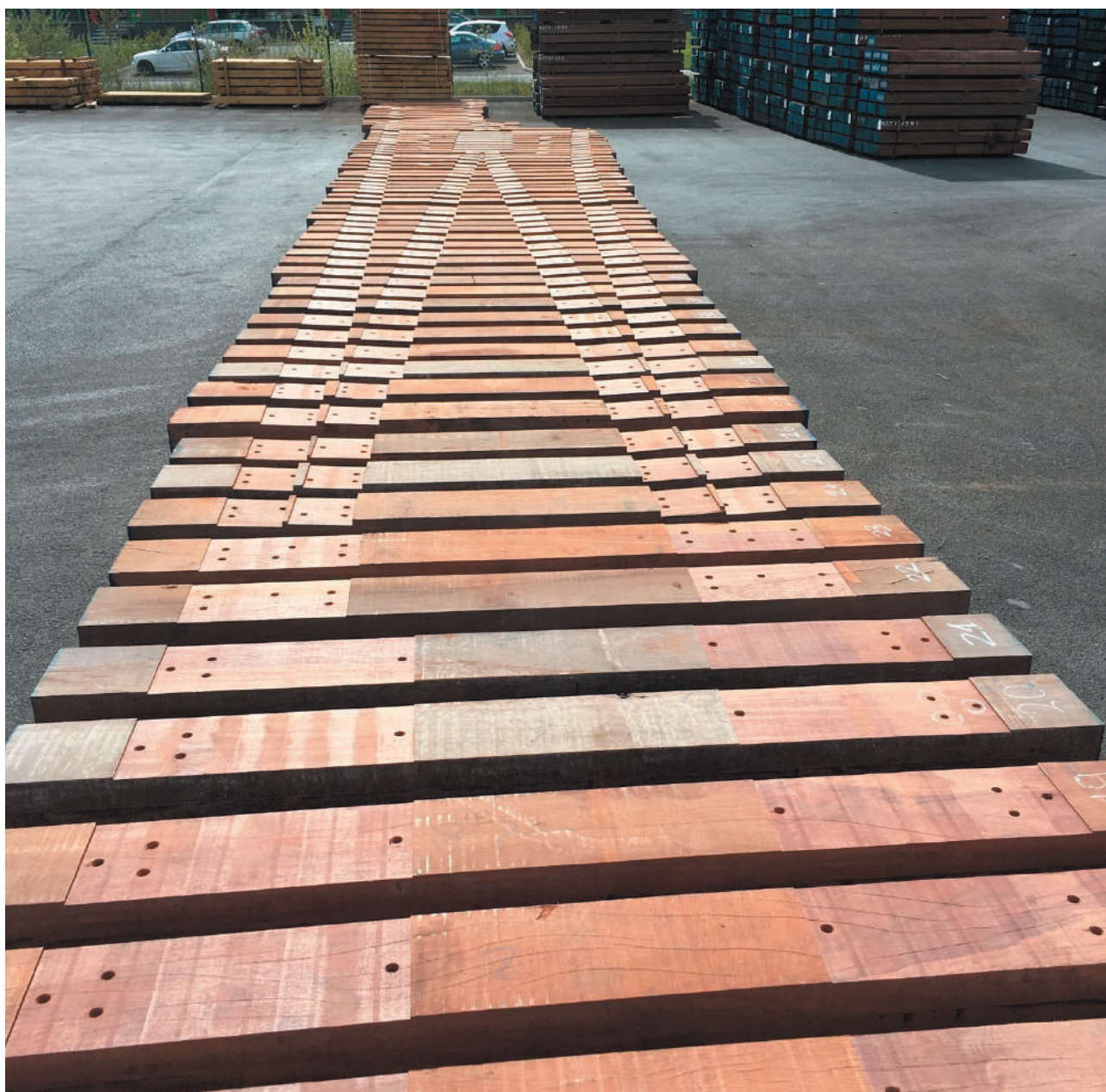
Shaping of Azobe pieces for railway switch and crossing layouts, RATP, Paris (photo Rail Europe)
