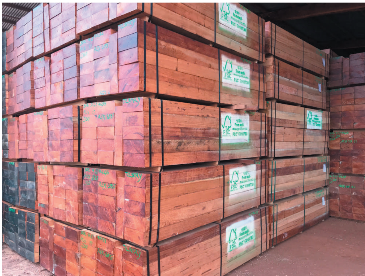
Sleepers made of Angelim (photo: Stéphane Glannaz, Mil Madeiras Preciosas Ltd. - Precious Woods Amazonas, Itacutiara, State of Amazonas, Brazil)
