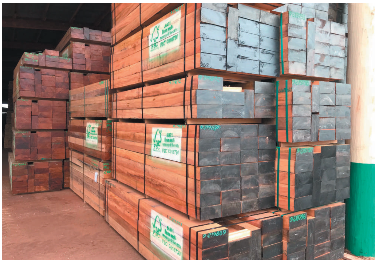
Sleepers made of Angelim and Angelim vermelho (in the back) (photo: Stéphane Glannaz, Mil Madeiras Preciosas Ltd. - Precious Woods Amazonas, Itacuatira, Amazonas State, Brazil)
